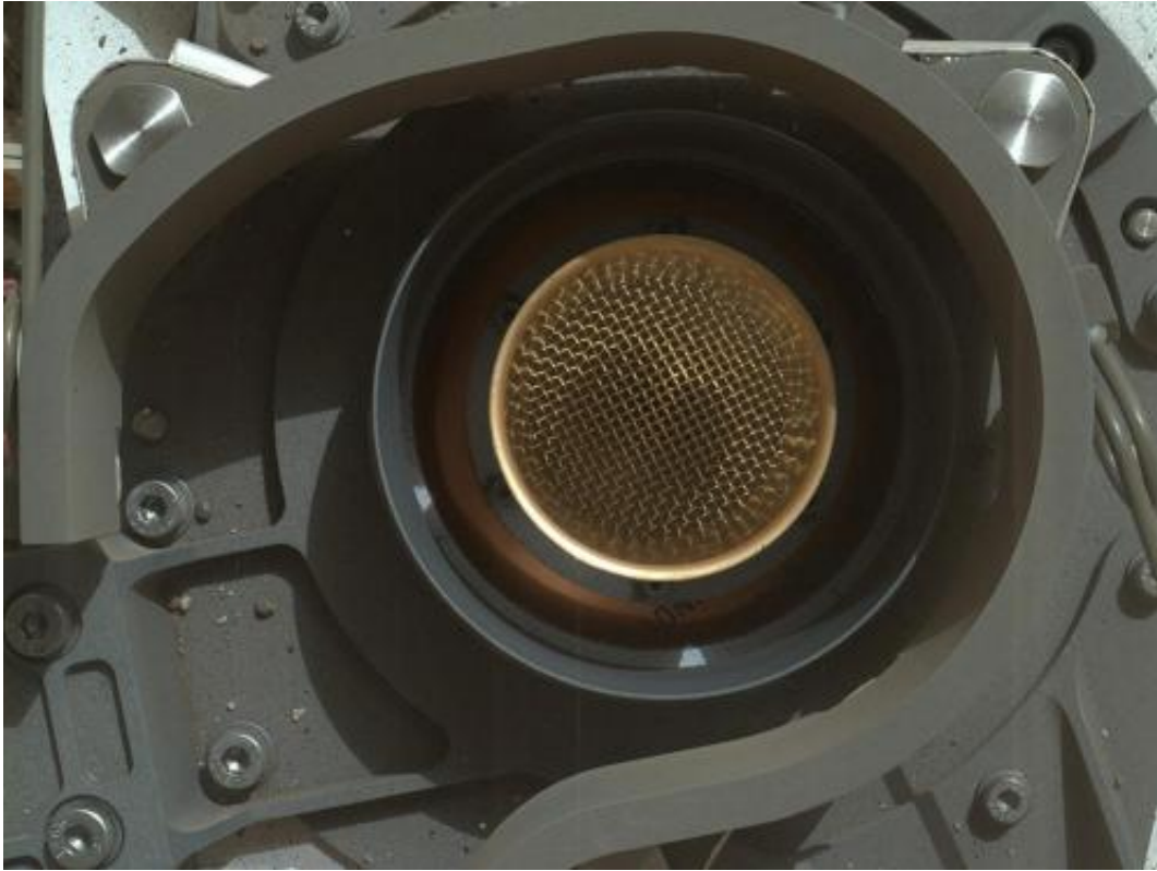
CheMin funnel for intaking samples of dirt and rock for analysis. Credit: NASA/JPL-Caltech/MSSS
