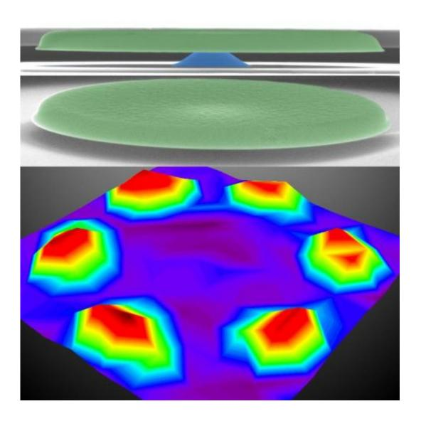
This image spatially maps and visualizes the shapes of multimode Brownian motions. The to of the image is a false-colored scanning electron micrographs of a silicon carbide (SiC) microdisk supported by a central pedestal made of 500nm-thick silicon oxide. The bottom image is a scanned map of vibrations of the
