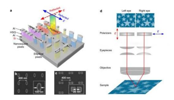
(Left) Elliptical and coupled nanosquare pixels scatter different wavelengths of light depending on polarization. (Right) The stereomicroscope setup uses different polarizers on each eyepiece to image two superposed microprints which contain pixels that present two laterally displaced images to the left and right eyes of a viewer, resulting in depth perception. Credit: Xiao Ming Goh, et al. ©2014 Macmillan Publishers Limited
