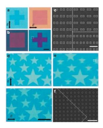
Microprints of a square and cross printed onto the same area formed from (a) elliptical nanopixels and (b) coupled nanosquare pixels under x- and y-polarized light. (c) SEM image of the region indicated by the dotted box in (b). (d) Images decoupled by polarizers. (e) Overlay of images in (d) to form a stereoscopic image with depth perception. (f) SEM image of the region indicated by the dotted box in (e). Credit: Xiao Ming Goh, et al. ©2014 Macmillan Publishers Limited
