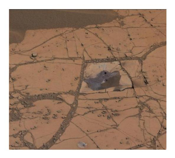
This image shows the first holes drilled by NASA's Mars rover Curiosity at Mount Sharp. The loose material near the drill holes is drill tailings and an accumulation of dust that slid down the rock during drilling. Credit: NASA/JPL-Caltech/MSSS
