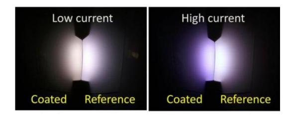
At low current the coated LEDs emit a cozy, warm glow compared to uncoated reference LEDs. Credit: Hugo J. Cornelissen
