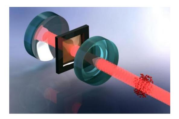
A cloud of ultracold atoms (red) is used to cool the mechanical vibrations of a millimeter-sized membrane (brown, in black frame). The mechanical interaction between atoms and membrane is generated by a laser beam and an optical resonator (blue mirror). Credit: Tobias Kampschulte, University of Basel
