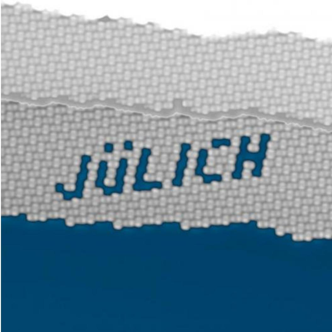
Jülich researchers 'stencilled' a word into a molecular monolayer by removing 47 molecules. Credit: Forschungszentrum Jülich
