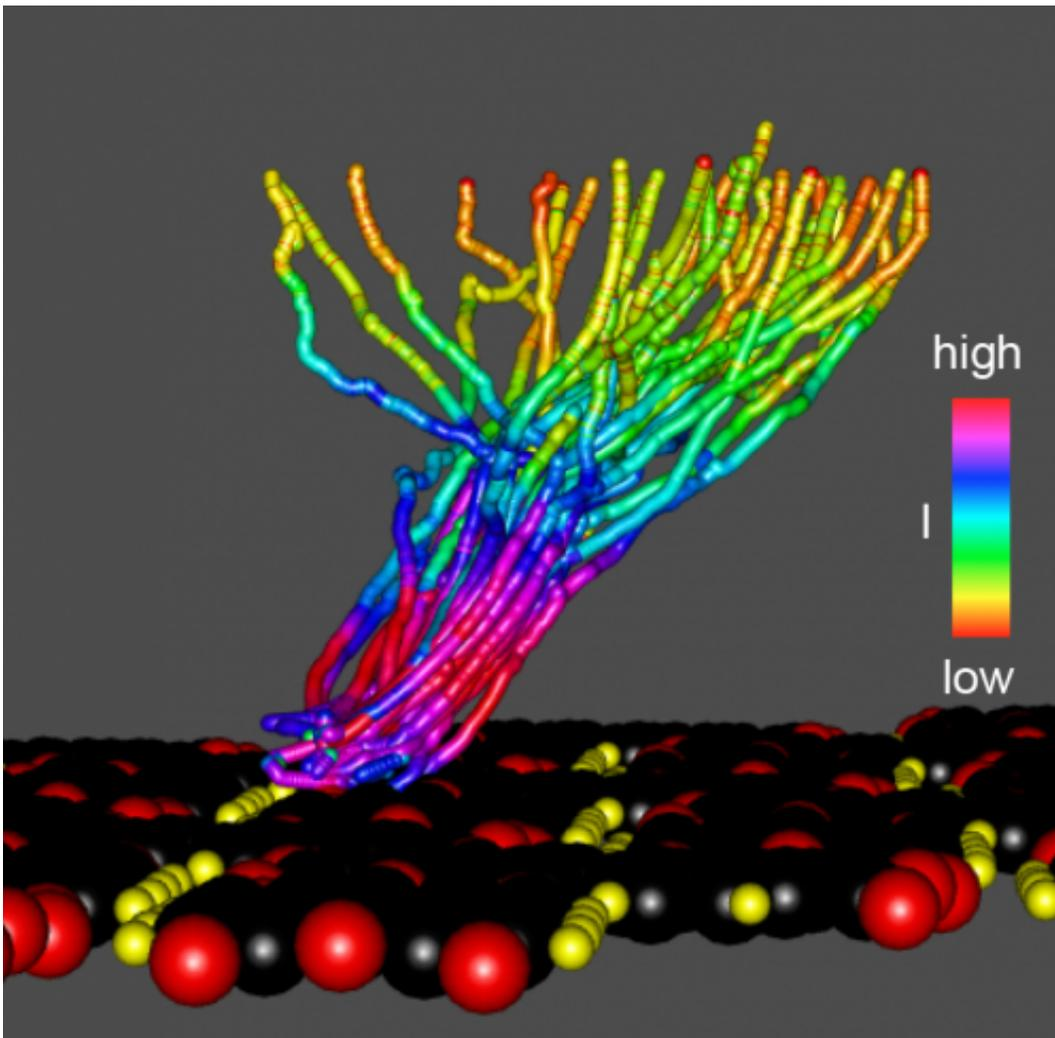
Entwined ways out: The molecules can be extracted by 'peeling' them from the layer, as shown by this image of the successful trajectories required to write 'JÜLICH'. Credit: Forschungszentrum Jülich
