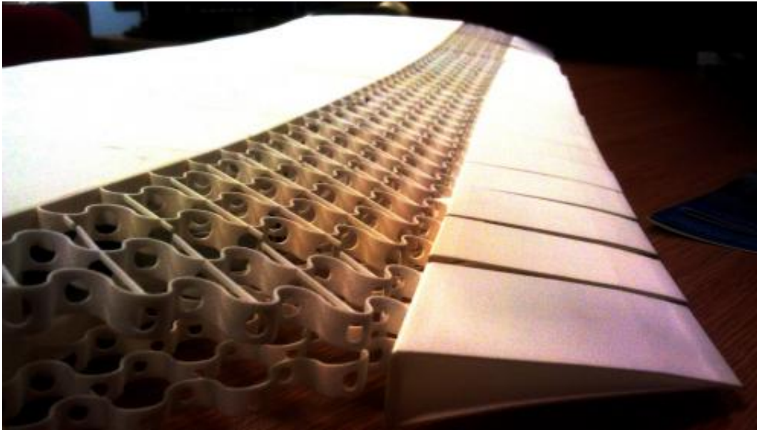
Skeleton of trailing edge of wing morphing wind-tunnel demonstrator concept Ash Dove-Jay, University of Bristol
