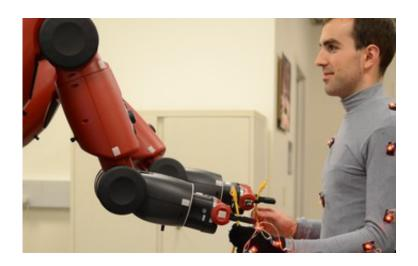
A sample experimental setup for human-robot object handoffs. Each experiment tested 30 randomly ordered handoffs, of which 10 each were generated using the constant, relative and personal schemes. The pose of the human test subject's torso was measured at the moment of the handoff using the eight motion capture markers on the chest and back. Credit: Aaron Bestick, UC Berkeley
