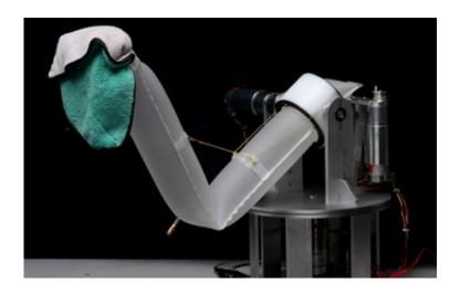
The inflatable arm has no rigid components in its structure and derives strength from pressurized air. The arm is actuated using, cables, motors and pneumatics. Credit: Sanan/CMU
