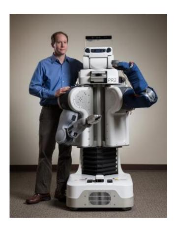
The blue cover on the arm of this robot protects an array of sensors that help it reach through the clutter of a typical home to perform personal care tasks. Charlie Kemp poses with the robot, which also holds an electric shaver. Credit: Rob Felt
