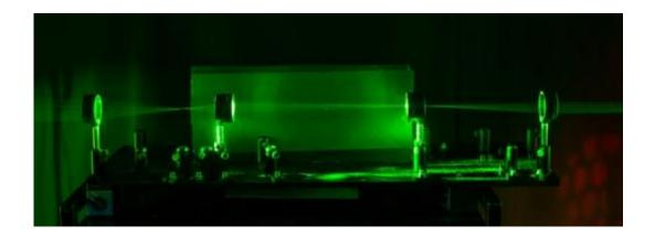
A side view. The laser shows the paths that light rays travel through the system, showing regions that can be used for cloaking an object. Credit: Adam Fenster / University of Rochester
