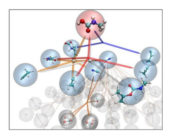
The nanoreactor works like a virtual chemistry set to discover new reactions and mechanisms. This diagram describes the reaction network for methylcarbamic acid, identifying all the reactions involving it or leading to its production. Credit: Todd Martinez
