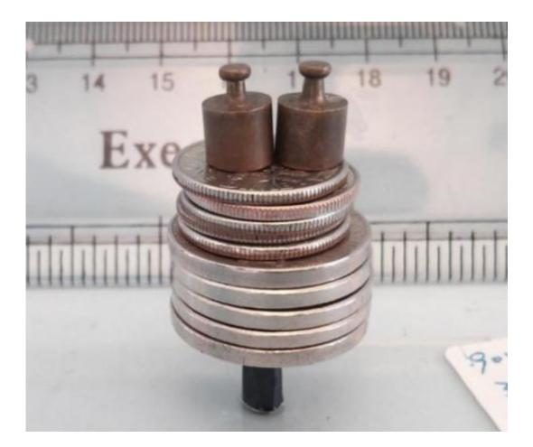
When rolled into a tube shape, the MXene-polymer nanocomposite exhibits excellent compressive strength. Credit: Drexel University
