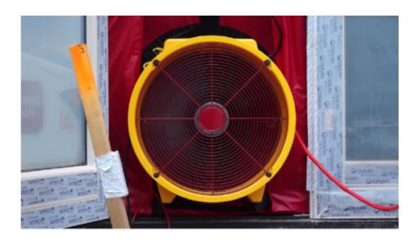
The airtightness of many Dutch homes will be determined thanks to researchers from the University of Twente. Based on more than one hundred reports of 'blower door tests' (which determine the airtightness of a home) that have been made available by companies, the University aims to make recommendations in the field of airtightness for municipalities and builders.
