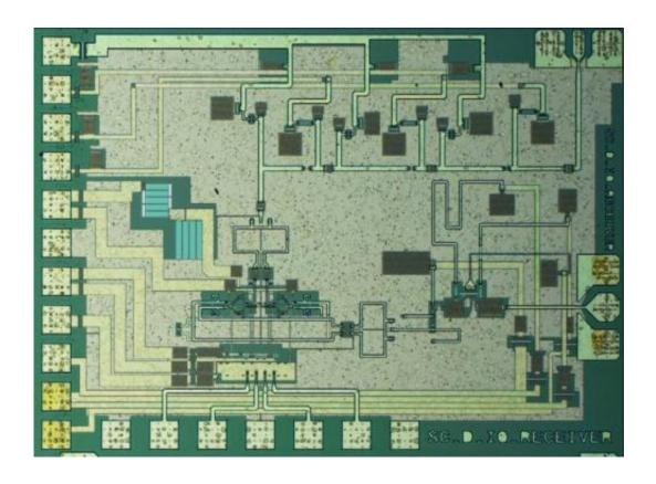
The photo shows the 140 GHz transmitter chip, containing an I-Q modulator, a 3-stage amplifier, and a x3 frequency multiplier for the local oscillator. The chip was designed by Sona Carpenter, Herbert Zirath, and Mingquan Bao. Data-transmission measurements was done by Simon He. The chip size is 1.6x1.2 mm2. Credit: Sona Carpenter
