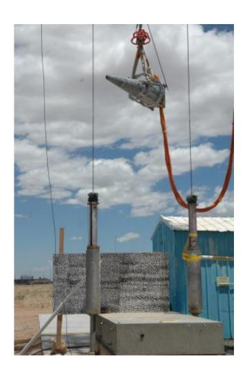
Sandia National Laboratories performed a drop test for the W88 ALT 370 program, designed to replicate a crane accidentally dropping the re-entry body onto a concrete surface. The test was conducted at Sandia's 185-foot Drop Tower Facility, using the same handling gear a crane would use to move the weapon.
