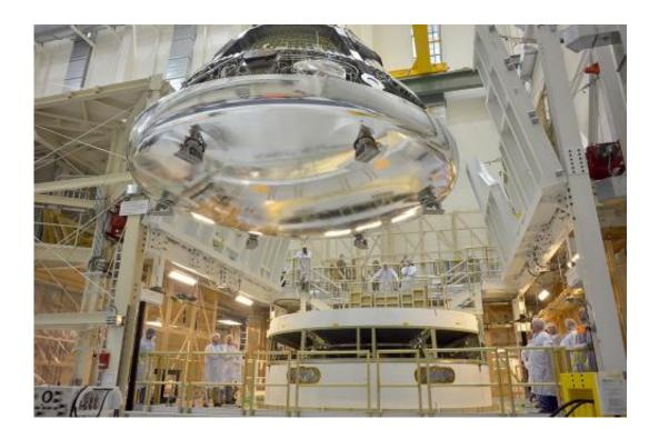
The Orion crew module for Exploration Flight Test-1 is shown in the Final Assembly and System Testing (FAST) Cell, positioned over the service module just prior to mating the two sections together. Credit: NASA/Rad Sinyak
