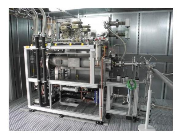
Researchers at a new hot gas test facility are testing the waste heat use systems and turbo-chargers. Their goal is to develop more efficient powertrain concepts for passenger vehicles and trucks. Credit: Fraunhofer ICT
