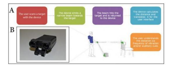
A flow chart depicting the use of the device and an illustration of a user. Note the two sensor beams, one pointing directly ahead, and one pointing towards the ground for obstacle detection. Credit: Restorative Neurology and Neuroscience
