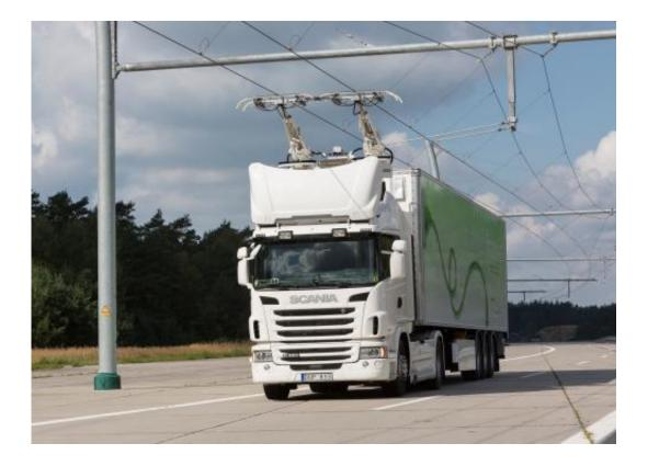
In the follow-up project, ENUBA 2, Siemens entered into a partnership with Scania, a Swedish company. The focus is on optimizing the integration of the drive system and pantograph into the vehicle and on providing the necessary traffic control systems. The picture shows a driving scene at the extended eHighway test track in Groß Dölln, Germany.
