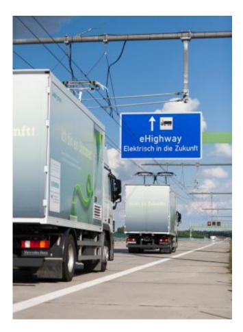
In the follow-up project, ENUBA 2, Siemens entered into a partnership with Scania, a Swedish company. The focus is on optimizing the integration of the drive system and pantograph into the vehicle and on providing the necessary traffic control systems. The picture shows a driving scene at the extended eHighway test track in Groß Dölln, Germany
