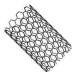
A team led by the Lawrence Livermore scientists has created a new kind of ion channel based on short carbon nanotubes, which can be inserted into synthetic bilayers and live cell membranes to form tiny pores that transport water, protons, small ions and DNA.
