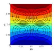
Flow pattern 2 min after the start of vibrations. Credit: © Y. Gaponenko et al.
