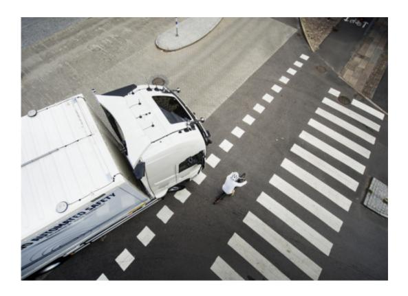
If the driver does not respond to the actions suggested by the system, the steering or braking system can be activated autonomously.
