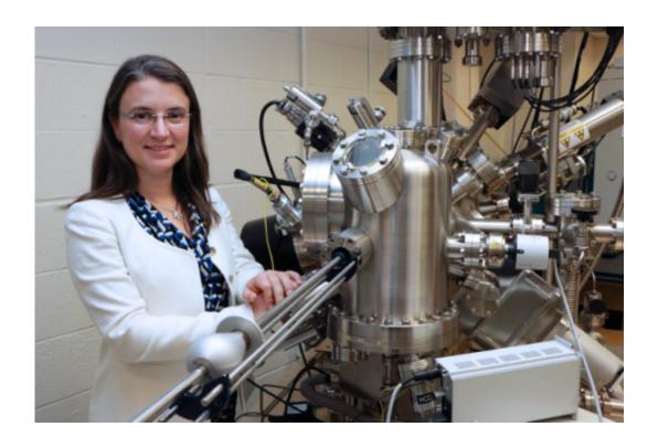
Bilge Yildiz with a scanning tunneling microscope customized to study oxide material surfaces at high temperatures under mechanical stress in the presence of oxygen, water vapor, or other reactive gases. Credit: Denis Paiste/Materials Processing Center
