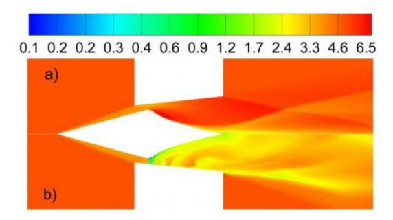
The effectiveness of current laser-propulsion techniques is limited by the instability of supersonic gas flow, caused by shock waves that "choke" the inlet of the nozzle, reducing thrust. Those effects can be reduced with the help of laser ablation, redirecting the plasma plume so that it flows close to the interior walls of a supersonic nozzle and significantly improving the overall thrust. Credit: Y.Rezunkov/IOIE
