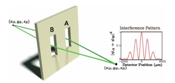
Two-slit experiment. Inset shows a typical interference pattern obtained by assuming  $\psi AB = \psi A + \psi B$ . Credit: Source: R. Sawant, J. Samuel, A. Sinha, S. Sinha, and U. Sinha, Nonclassical Paths in Quantum Interference Experiments, *Phys. Rev. Lett.* 113, 120406 (2014).
