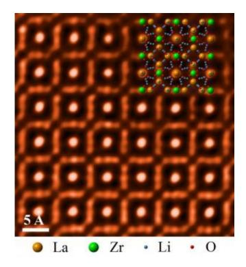
ORNL researchers used scanning transmission electron microscopy to take an atomic-level look at a cubic garnet material called LLZO that could help enable higher-energy battery designs. Credit: ORNL
