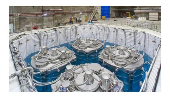
Antineutrino detectors in Daya Bay Hall #3. The detectors rest in a pool being filled with ultrapure water. Credit: University of California - Lawrence Berkeley National Laboratory
