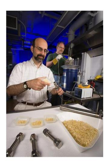
Biochemical engineer Bruce Dien and microbiologist Loren Iten use mini-batch reactors to pretreat biomass at high temperatures to prepare it for fermentation to ethanol. Here, they are pretreating corn fiber, but the process is the same for switchgrass. Credit: Peggy Greb
