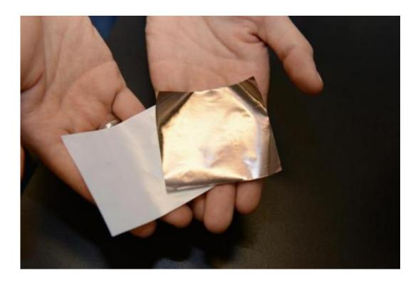
Stanford scientists have developed a lithium-ion battery that alerts users of potential overheating and fire. The early-warning system uses an ultrathin copper sensor deposited atop a conventional battery separator (white square). Credit: Mark Shwartz, Precourt Institute for Energy, Stanford University
