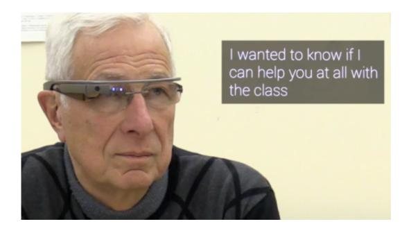
A hard-of-hearing person wears Glass while a second person speaks directly into a smartphone. The speech is converted to text, sent to Glass and displayed on its heads-up display. Credit: Georgia Tech
