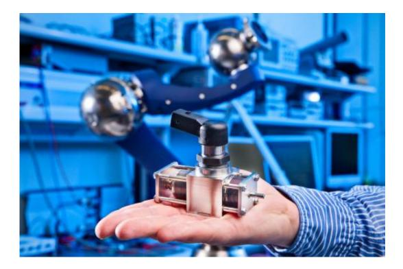
Researchers at Siemens have developed a small but powerful piezohydraulic actuator. Although it is only about nine centimeters long, it can apply a force of more than 150 newtons — equivalent to a weight of 15 kilograms. Such actuators are used to operate valves and flaps, for example, and can also be employed in robots.
