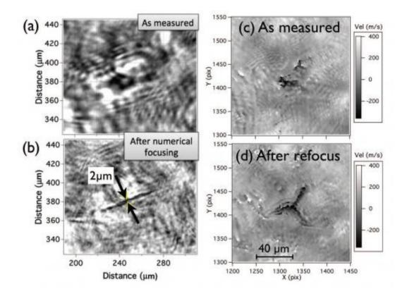
In a recent article published in the *Review of Scientific Instruments*, a research team led by scientists at Lawrence Livermore National Laboratory describe a technique for 3D-image processing of a high-speed photograph of a target, "freezing" its motion and revealing hidden secrets.
