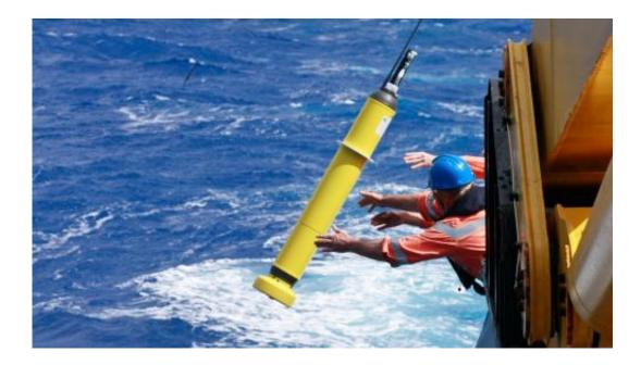
Akin to having a fleet of miniature research vessels, the global flotilla of more than 3,600 robotic profiling floats provides crucial information on upper layers of the world's ocean currents. Credit: Alicia Navidad/CSIRO.
