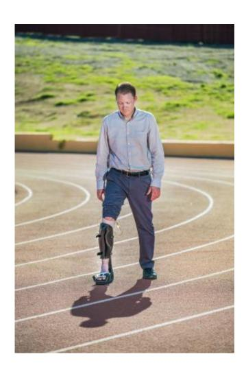
Sandia National Laboratories researcher Jason Wheeler demonstrates a special clamp-on socket with an artificial foot that helps him test a liner Sandia is developing for prosthetics. The two-piece socket shifts the load from Wheeler's foot to his leg, giving him a better idea of what an amputee feels. Credit: Randy Montoya
