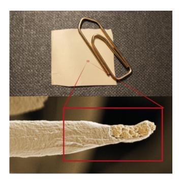
A close-up of the antibacterial fibre created by the KTH scientists. In this 2x2cm swatch of fabric are nearly 200,000 threads running in the same direction.
