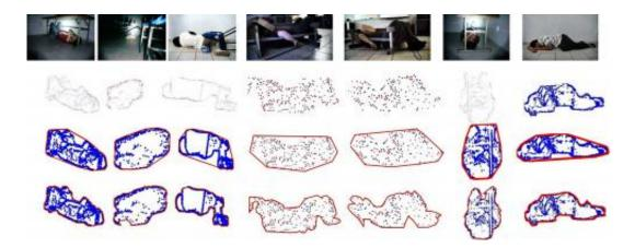
Once the robot obtains silhouettes, it uses the descriptor system that obtains the visual characteristics (3D points) to segment (wrapping objects in circles) and then builds the human external silhouettes. These silhouettes will serve as descriptors to train a <u>neural network</u> called CSVM, developed by Arana Daniel, to recognize patterns
