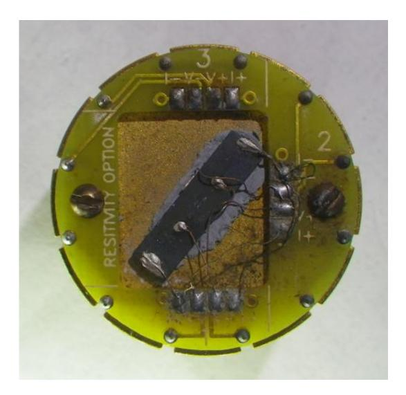
Researchers at Caltech devised a way to calculate the electrical properties of individual components of a composite material by testing the material's response in a range of magnetic fields. This image shows the material wired in a sample holder designed to measure its electrical properties. Credit: Tristan Day/Caltech
