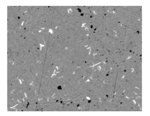
The multi-phase thermoelectric Cu(1.97)Ag(0.03)Se consists of a main crystal structure of Cu(2)Se and an impurity phase with the crystal structure of CuAgSe. In this scanning electron microscope image the impurity phase shows up as light spots. The dark spots are voids in the crystal structure. Credit: Tristan Day/Caltech
