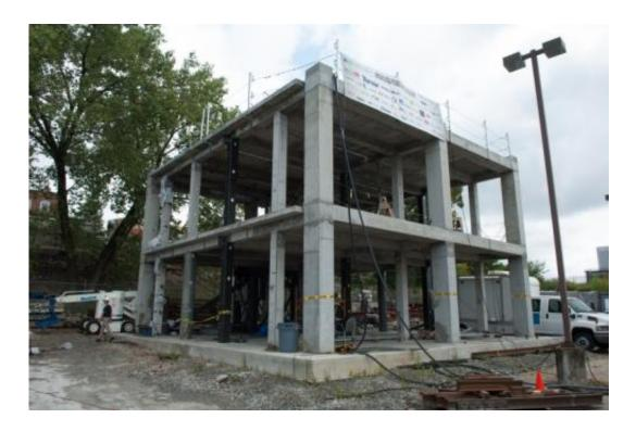
"It is a full-scale building that was constructed from plans of a building that was built in the 1950s in California," DesRoches said. "We know exactly what is in the columns and how it was designed."
