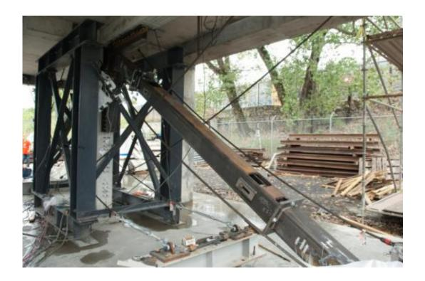
The third and final retrofit uses a "smart" material known as a shape-memory alloy. It can deform significantly and then revert to its original shape. "You can bend it, and it does not break," DesRoches said. "The idea behind seismic retrofit is that you want the structure to bend, but not break. So we have these braces and shape-memory alloy cables in this brace, and when it deforms, it puts the force right back on the structure to pull it back into position."
