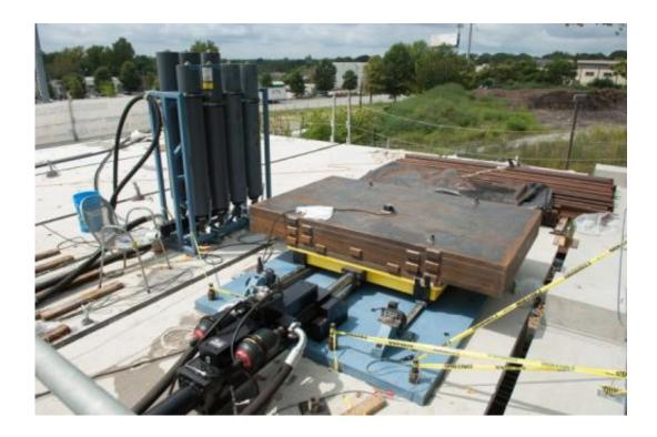
Researchers mounted a shaker on top of each research bay, clamping it down to the building. This shaker produced more than 100,000 pounds of force, and researchers could control the sort of harmonic load or non-harmonic load needed. "Nobody has really tested anything at this scale the way we are testing it with a large-scale shaker on top of the building," DesRoches said. "From a technical perspective, this is very unique."
