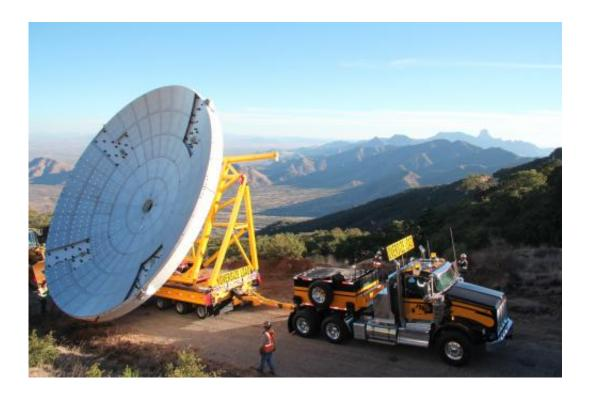
With the new antenna in tow, a special haul truck crawls up the winding road to Kitt Peak. Credit: Lucy Ziurys
