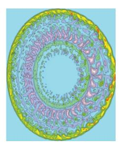
Supercomputer simulation shows turbulent density fluctuations in the core of the Alcator C-Mod tokamak during strong electron heating. Credit: D. R. Ernst, MIT
