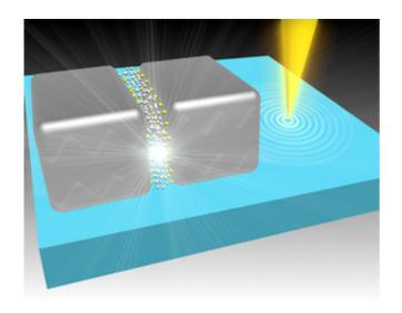
An electron nanoprobe (yellow) placed near the functionalized silver nanoparticles measured plasmon-assisted quantum tunneling at terahertz frequencies. Credit: Shu Fen Tan, National University of Singapore
