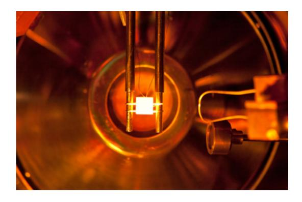
Lithium-coated molybdenum was heated to a high temperature during a PPPL experiment. Credit: Angela Capece, PPPL
