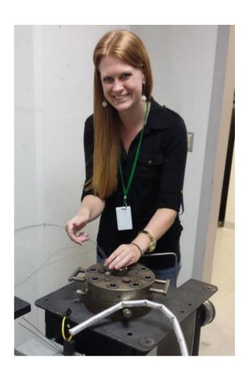
Erika Kohler places thermocouples into a pressure chamber at NASA's Goddard Space Flight Center. The thermocouples measure the temperature of the chamber to ensure it reaches Venusian temperatures.
