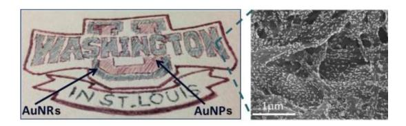
A hand drawing of Washington University logo using gold nanorods (AuNRs) and gold nanospheres (AuNPs) as plasmonic ink, in which red and green colors result from the inherent optical properties of nanopaticles (Right: A representative scanning electron microscopy image of gold nanorods on paper). Credit: L.Tian/WU
