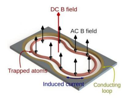
Shaped atom-chip microtrap comprised of a conducting loop (gold) in which currents are induced in the same way as a transformer.
