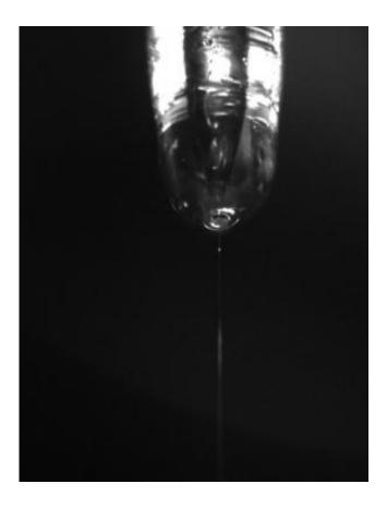
This is a microscope image of the liquid jet in vacuum. The glass nozzle you see there has a diameter of 1 mm and the thin liquid jet coming out from the nozzle has a diameter of only 20  $\mu$ m. Credit: S. Schreck, HZB/UP
