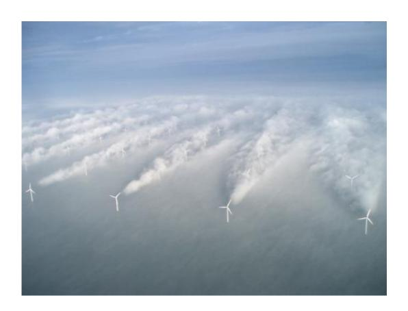
Wind parks produce their own air circulation dynamics. First row turbines get more wind than those in the middle. They also produce vortices that affect the performance of downstream turbines. Learning software can reduce these effects by optimizing rotor speeds and blade angles.
