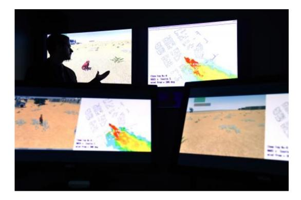
Adam Moses of the U.S. Naval Research Laboratory (NRL) was asked to build a program for handlers of improvised explosive device (IED)-detecting dogs to train in a virtual environment, because of NRL's expertise with modeling plumes for hazardous material releases and attacks in urban environments. "[An IED is] actually leaking all this gas subtly, that no human built sensor could read because the particles are so small," says Moses. "Per billion is the level these dogs can
