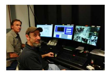
NIST's new calibration service for high-power lasers is controlled from behind a protective barrier. The laser is monitored by a camera and is visible in the upper left corner of the right-hand screen. Paul Williams (left) and Joshua Hadler operate the service, which can calibrate lasers with up to 10 kilowatts of power for manufacturers and military customers. Credit: Burrus/NIST
